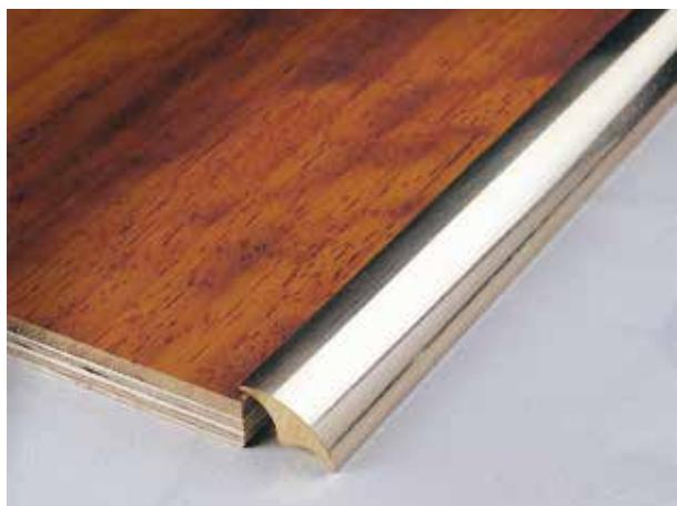
VARIOTEC DC profiles' innovative design elegantly rotates and adapts to match different floor elevations. By simply rotating its shape, this profile can adapt to floor thicknesses ranging from 7 to 14mm. Use our adhesive for on-site installation.
